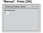
Using the Number buttons or [▲ / ▼], enter your PBS channel number. Press [OK]. The setting will be activated.
